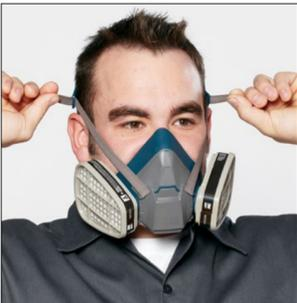
Pull the ends of the straps to adjust the tightness, beginning with the adjustment points on the head cradle and then moving to the adjustment points at the back of the neck. Do not over-tighten. Strap tension may be decreased by pushing out on back side of buckles.
